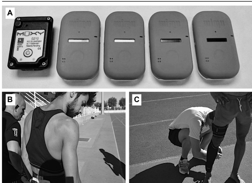
Figure 1. WIMU PRO inertial devices and MOXY NIRS unit used in this research (A) before placing in the auto-calibration process, (B) scapulae device location with a specific harness and COM unit location using elastic adhesive band, and (C) ankle and knee device location using elastic adhesive band and NIRS unit location using a compression garment. COM = center of mass; NIRS = near-infrared spectroscopy.
